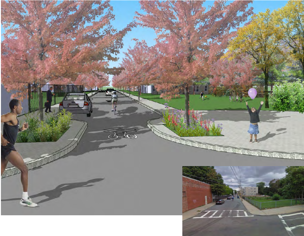
A Greenway Street (described on the following page) with widened sidewalks, bump outs on the corners for traffic calming, new open space and a shared bicycle/vehicular travel lane. The existing condition is shown on the inset.
